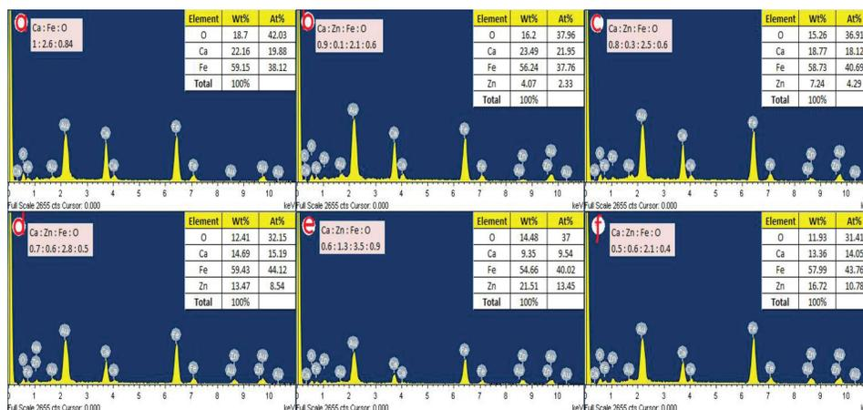
**Figure 6.** EDX of bulk material. (a)  $\text{CaFe}_2\text{O}_4$  (b)  $\text{Ca}_{0.9}\text{Zn}_{0.1}\text{Fe}_2\text{O}_4$  (c)  $\text{Ca}_{0.8}\text{Zn}_{0.2}\text{Fe}_2\text{O}_4$  (d)  $\text{Ca}_{0.7}\text{Zn}_{0.3}\text{Fe}_2\text{O}_4$  (e)  $\text{Ca}_{0.6}\text{Zn}_{0.4}\text{Fe}_2\text{O}_4$  (f)  $\text{Ca}_{0.5}\text{Zn}_{0.5}\text{Fe}_2\text{O}_4$ .
