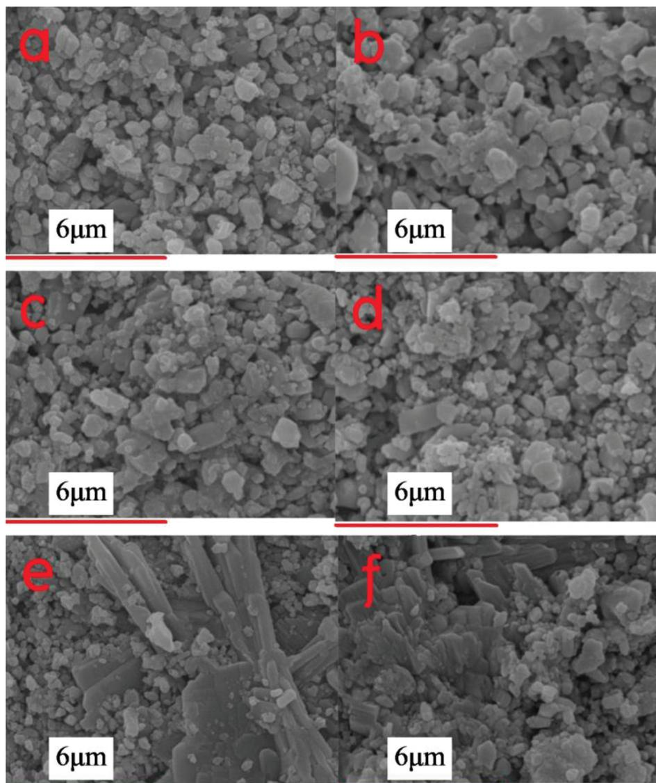
**Figure 5.** The microstructure of bulk material (a)  $\text{CaFe}_2\text{O}_4$  (b)  $\text{Ca}_{0.9}\text{Zn}_{0.1}\text{Fe}_2\text{O}_4$  (c)  $\text{Ca}_{0.8}\text{Zn}_{0.2}\text{Fe}_2\text{O}_4$  (d)  $\text{Ca}_{0.7}\text{Zn}_{0.3}\text{Fe}_2\text{O}_4$  (e)  $\text{Ca}_{0.6}\text{Zn}_{0.4}\text{Fe}_2\text{O}_4$  (f)  $\text{Ca}_{0.5}\text{Zn}_{0.5}\text{Fe}_2\text{O}_4$ .
