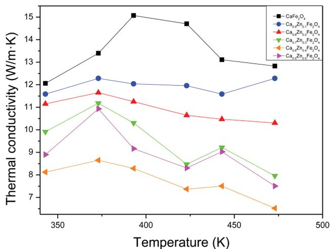
**Figure 7.** The relationship of thermal conductivity and temperature for  $\text{Ca}_{1-x}\text{Zn}_x\text{Fe}_2\text{O}_4$  (where  $x = 0.0-0.5$ ).
