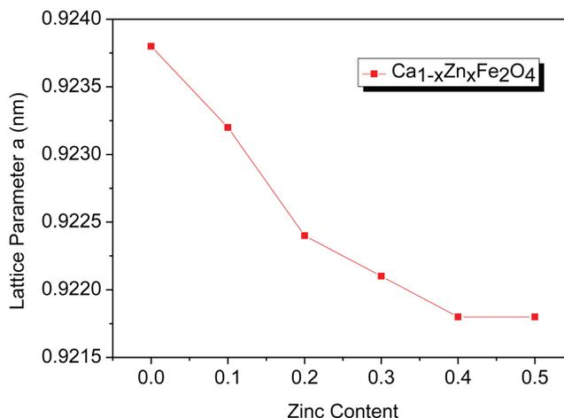
**Figure 3.** The relationship of lattice parameter  $a$  with zinc content: Ca<sub>1-x</sub>Zn<sub>x</sub>Fe<sub>2</sub>O<sub>4</sub> (where x = 0.0–0.5).
