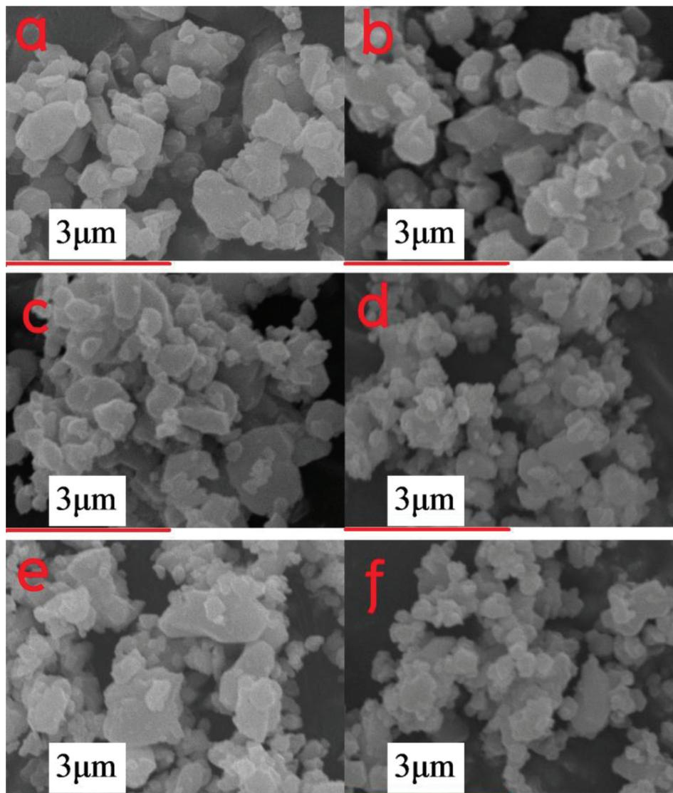
**Figure 4.** The microstructure of powder material. (a)  $\text{CaFe}_2\text{O}_4$  (b)  $\text{Ca}_{0.9}\text{Zn}_{0.1}\text{Fe}_2\text{O}_4$  (c)  $\text{Ca}_{0.8}\text{Zn}_{0.2}\text{Fe}_2\text{O}_4$  (d)  $\text{Ca}_{0.7}\text{Zn}_{0.3}\text{Fe}_2\text{O}_4$  (e)  $\text{Ca}_{0.6}\text{Zn}_{0.4}\text{Fe}_2\text{O}_4$  (f)  $\text{Ca}_{0.5}\text{Zn}_{0.5}\text{Fe}_2\text{O}_4$ .
