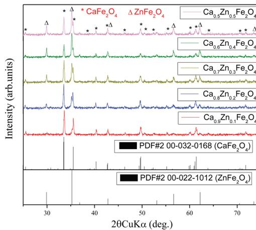
Figure 2. XRD patten of the  $\text{Ca}_{1-x}\text{Zn}_x\text{Fe}_2\text{O}_4$  (where  $x = 0.0-0.5$ ).
