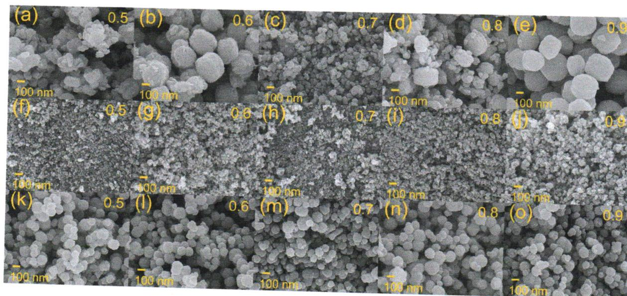
Fig. 1 SEM images of ZNPs synthesized at 65 °C (a-e), 75 °C (f-j) and 85 °C (k-o).
