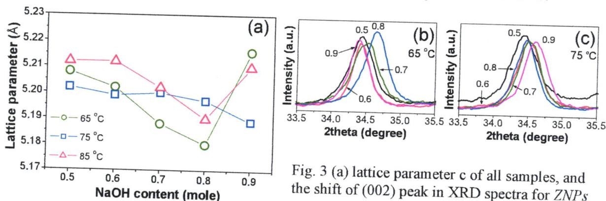
Fig. 3 (a) lattice parameter  $c$  of all samples, and the shift of (002) peak in XRD spectra for *ZNPs* synthesized at (b) 65 °C and (c) 75 °C.
